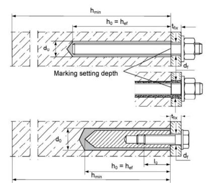
fischer threaded rod pre-positioned anchorage
